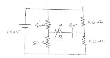
(b) Calculate the branch current I, and I<sub>2</sub> for the circuit shown in Figure.
